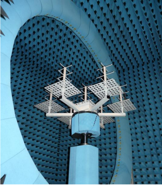
Figure 7: Measurement of final antenna in SATIMO SG-64 multiprobe spherical near field range.
