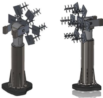
Figure 3: Galileosat ground station antenna on the dedicated positioner
